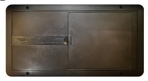
All circuits and equipment in the coach area of the van are protected by either a fuse panel or breaker panel. When a circuit is overloaded or a "short" develops in any part of the system, a fuse or breaker will shut down that circuit. If this happens, turn off all affected lights or appliances and reset the breaker or replace the fuse with a new one of equal amperage rating.
