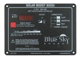
Shows battery voltage, input/output charge current, solar charge amp hours or auxiliary output voltage. The red AMP indicator light will be solid for output current or blinking for PV input current.
