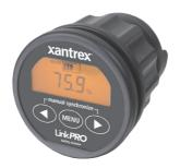
The LinkPRO can measure currents up to 10,000 Amps. It selectively displays voltage, charge and discharge current, consumed amp hours, remaining battery capacity and the time remaining of your battery bank.
